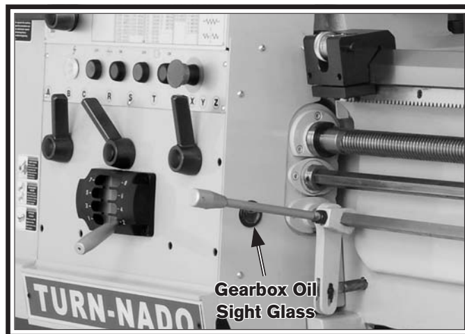
Figure 99. Location of quick-change gearbox oil sight glass.
